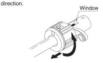
**4. Pull the TKS off of the tubing to complete stripping.** The tube can be attached as it is to a FR One-touch fitting.
