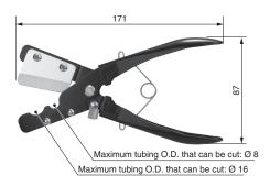
Note) Do not use it to cut the metalic materials such as electric wires.
