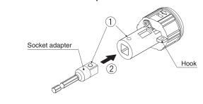
Connection with tools such as an air driver is also possible. Note) Ensure the TKS does not shake or vibrate.
